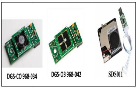
Figure 2: CO, O<sub>3</sub>, and Suspended Particle Sensors.
